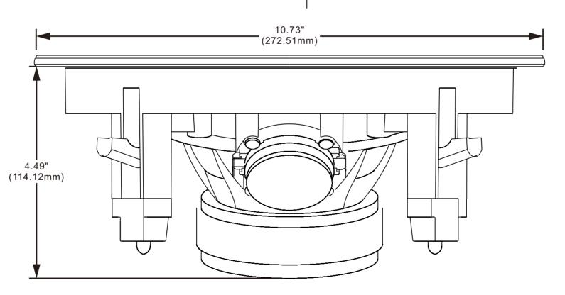
Note: 1" (25.4mm) must be clear behind the drywall to provide adequate room for the mounts to engage.
